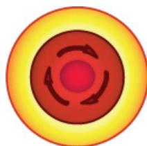
If you press Emergency Stop button on the machine operator's manual, machine movement stops in a moment. This button is locked when it is pressed, and can be unlocked by twisting it CW.
