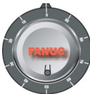
When Handle mode is selected, clockwise (CW) rotation of the handwheel gives positive axis motion, counterclockwise (CCW) rotation will give negative axis motion. When in Handle mode, both axis selection and incremental distance moved, are made using the selection and increment pushbuttons on the Operator Panel A. The increments are:
