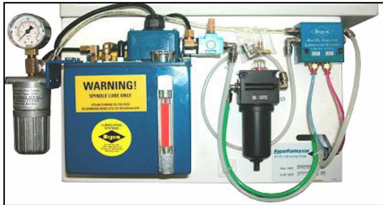
Figure 1-1: Spindle oil reservoir (optional)
