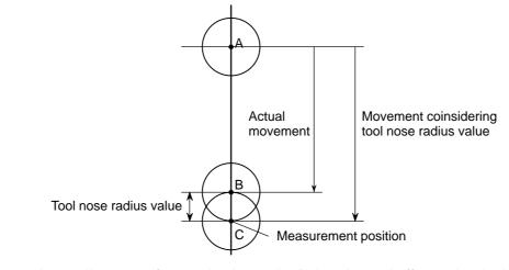
The tool actually moves from point A to point B, but the tool offset value is determined assuming that the tool moves to point C considering the tool nose radius value.
