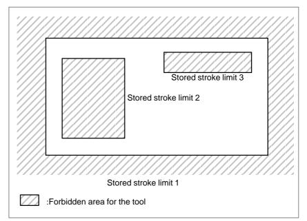
Fig. 6.3 (a) Stroke check
