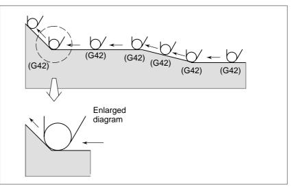
Tool movement when the workpiece position changes
