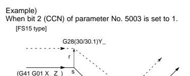
2 When a G28, G30, or G30.1 command is specified as a start–up block, a vector perpendicular to the direction in which the tool moves is created at the intermediate position. The vector is then canceled at the reference position. The next block creates an intersection vector.
