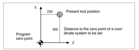
Fig. 1.3.2 (b) Coordinate system specified by the CNC
