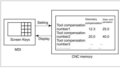
Fig. 1.6 (b) Displaying and Setting Offset Values
