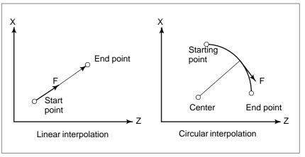
Fig. 5.3 (a) Tangential feedrate (F)
