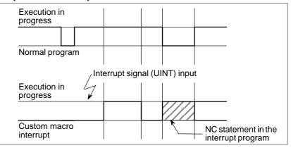
• Conditions for enabling and disabling the custom macro interrupt signal The interrupt signal becomes valid after execution starts of a block that contains M96 for enabling custom macro interrupts. The signal becomes invalid when execution starts of a block that contains M97. While an interrupt program is being executed, the interrupt signal becomes invalid. The signal become valid when the execution of the
