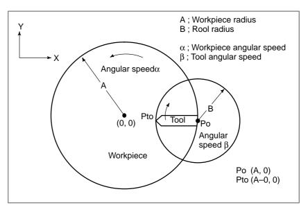
In this case, the tool nose position Pt (Xt, Yt) after time t is expressed by equation 1:
