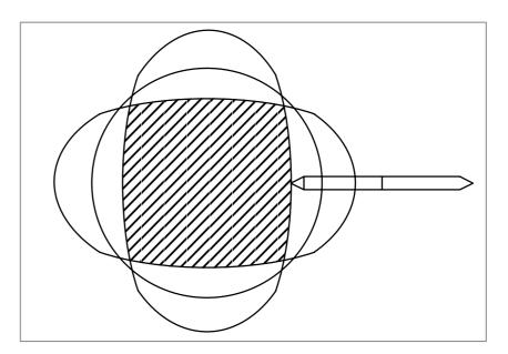
If three tools are set at every  $120^{\circ}$ , the machining figure will be a hexagon as shown below.
