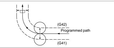
• Tool nose radius compensation when the block is specified from the MDI In this case, tool nose radius compensation is not performed.
