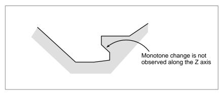
Fig. 13.2.1 (c) Figure Which Cannot Be Machined in Stock Removal in Turning (Type II)
