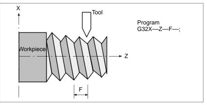
Fig. 1.1 (f) Taper thread cutting
