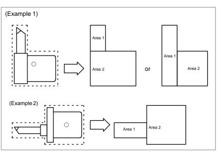
The coordinates of the upper and lower ends (points A and B shown below) of each of two rectangles are set, with the reference point of the tool post set as the origin.
