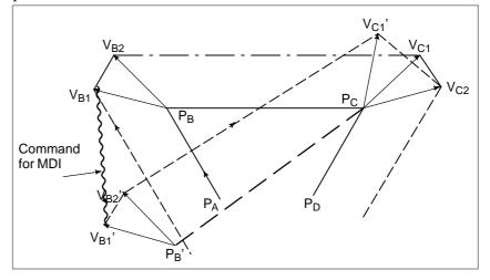
When position  $P_A$ ,  $P_B$ , and  $P_C$  are programmed in an absolute command, tool is stopped by the single block function after executing the block from  $P_A$  to  $P_B$  and the tool is moved by MDI operation. Vectors  $V_{B1}$  and  $V_{B2}$ are translated to  $V_{B1}$ ' and  $V_{B2}$ ' and offset vectors are recalculated for the vectors  $V_{C1}$  and  $V_{C2}$  between block  $P_B$ – $P_C$  and  $P_C$ – $P_D$ .
