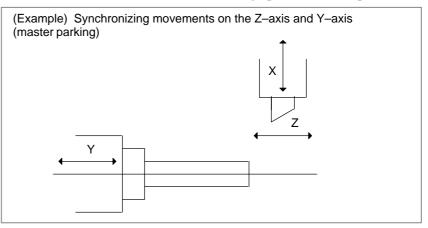
Movement is performed for the X-axis and Y-axis according to commands issued for the X-axis and Z-axis. (The Y-axis movement is synchronized with that of the Z-axis.) If the Z-axis is set to the parking state, the coordinates on the Z-axis and Y-axis are updated.
