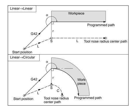
Tool movement around the outside of a corner at an obtuse angle (90° ≤ α<180°)</li>
