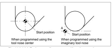
Fig. 14.2.1 (a) Tool nose radius center and imaginary tool nose
