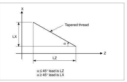
Fig. 4.8 (e) LZ and LX of a Tapered Thread
