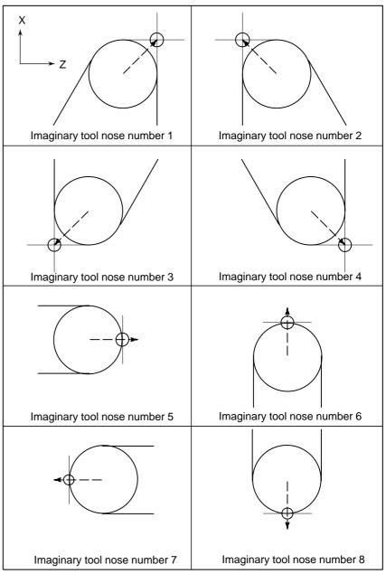
Fig. 14.2.2 Direction of imaginary tool nose
