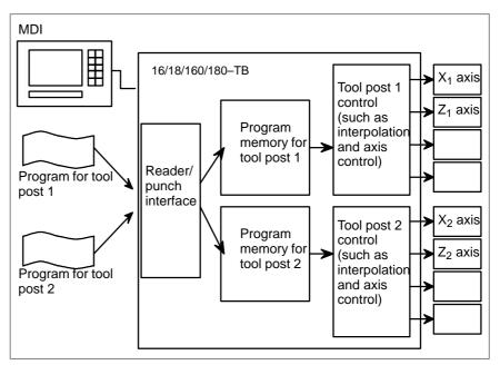
Fig. 20.1 (c) Controlling two tool posts independently at the same time
