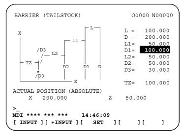
4 Position the cursor to each item defining the shape of the chuck or tailstock, enter the corresponding value, then press the [INPUT] soft key. The value is set. Pressing the [+INPUT] soft key after a value has been entered adds the entered value to the current value, the new setting being the sum of the two values.
