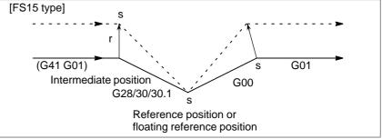
G28, G30, or G30.1 command in offset mode (with movement to a reference position not performed)
