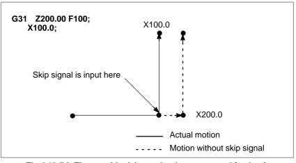
Fig.4.13 (b) The next block is an absolute command for 1 axis
