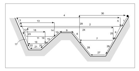
Fig. 13.2.1 (f) Cutting Path in Stock Removal in Facing
