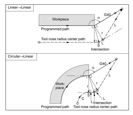
Tool movement around an outside corner at an acute angle (α<90°)</li>
