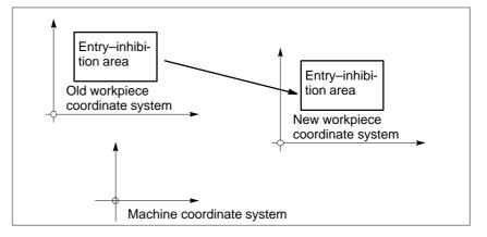
Use of the following commands and operations will shift the workpiece coordinate system.
