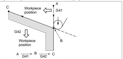
Although the workpiece does not exist on the right side of the programmed path in the above case. the existence of the workpiece is assumed in the movement from A to B. The workpiece position must not be changed in the block next to the start–up block. In the above example, if the block specifying motion from A to B were the start–up block, the tool path would not be the same as the one shown.
