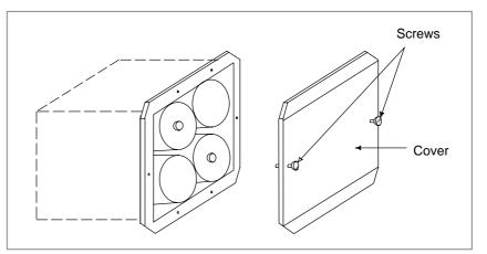
(4) After installing the new batteries, replace the cover.
