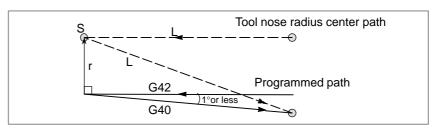
When a block without tool movement is commanded together with an offset cancel, a vector whose length is equal to the offset value is produced in a normal direction to tool motion in the earlier block, the vector is cancelled in the next move command.
