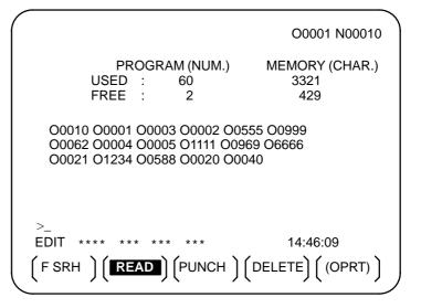
4 To specify a program number to be assigned to an input program, enter address O, followed by the desired program number. If no program number is specified, the program number in the file or on the NC tape is assigned as is.
