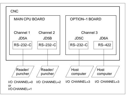
This CNC has three channels of reader/punch interfaces. The input/output device to be used is specified by setting the channel connected to that device in setting parameter I/O CHANNEL.
