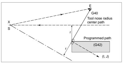
When an intersection is not obtainable, the tool comes to the normal position to the previous block at the end of the previous block.
