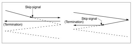
2. The skip signal is valid during dwell, without being affected by parameters DS1 to DS8 (No. 6206#0 to #7). Dwell is immediately stopped for return to the Z axis coordinate where the cycle started.
