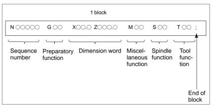
Fig. 1.7 (b) Block configuration
