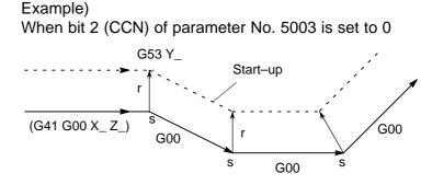
2 When a G53 command is specified as a start-up block, the next block actually becomes the start-up block. When bit 2 (CCN) of parameter No. 5003 is set to 1, however, the next block creates an intersection vector.
