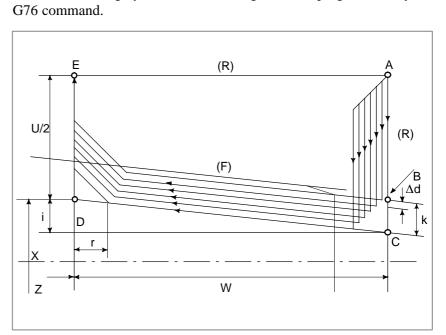
The thread cutting cycle as shown in Fig.13.2.7 is programmed by the
