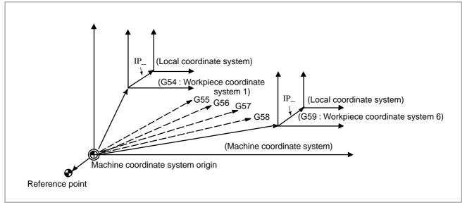
Fig. 7.3 Setting the local coordinate system
