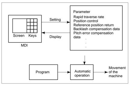
Fig. 1.6 (e) Displaying and setting parameters
