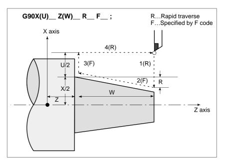
Fig. 13.1.1 (b) Taper Cutting Cycle
