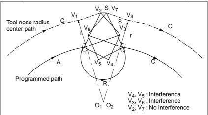
(Example 2) The tool moves linearly from V<sub>1</sub>, V<sub>2</sub>, V<sub>7</sub>, to V<sub>8</sub>
