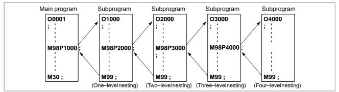
A single call command can repeatedly call a subprogram up to 9999 times. For compatibility with automatic programming systems, in the first block, Nxxxx can be used instead of a subprogram number that follows O(or:). A sequence number after N is registered as a subprogram number.
