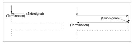
3. The skip signal is valid during dwell, without being affected by parameters DS1 to DS8 (No. 6206#0 to #7). Dwell is immediately stopped for return to the Z axis coordinate where the cycle started.
