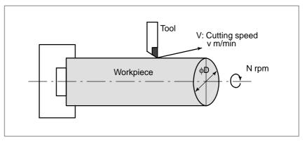
Fig. 1.4 Cutting speed
