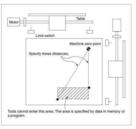
Besides strokes defined with limit switches, the operator can define an area which the tool cannot enter using a program or data in memory. This function is called stroke check.
