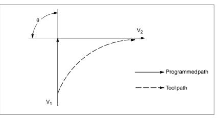
Fig. D.3 (a) Slight deviation between the tool path and the programmed path
