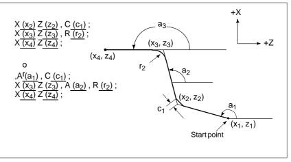
Fig. 13.7 Machining Drawing (example)
