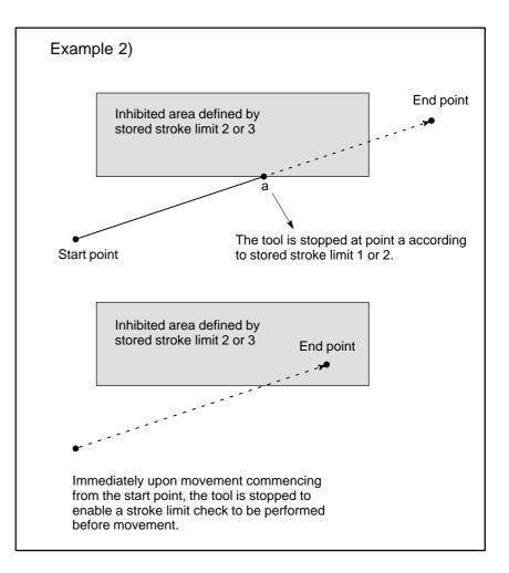
When a stroke limit check prior to movement is performed, whether to check the movement performed by a G31 (skip) block and G37 (automatic tool length measurement) block can be determined using NPC (bit 2 of parameter No. 1301).
