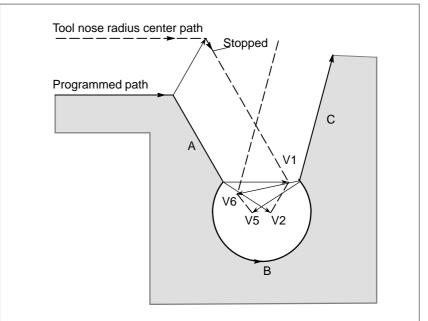
After ignoring vectors  $V_2$  and  $V_5$  because of interference, interference also occurs between vectors  $V_1$  and  $V_6$ . The alarm is displayed and the tool is stopped.
