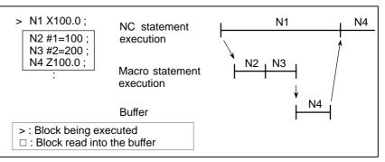
When N1 is being executed, the next NC statement (N4) is read into the buffer. The macro statements (N2, N3) between N1 and N4 are processed during execution of N1.
