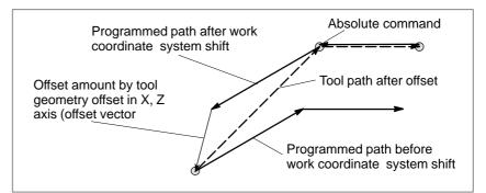
Fig. 14.1.5 (c) Movement of tool geometry offset
