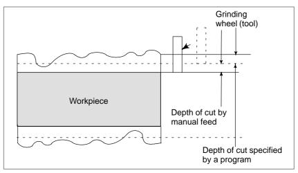
Fig. 1.3 (c) Handle Interruption for Automatic Operation
