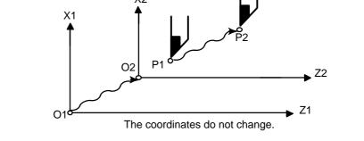
Fig. 3.5 (b) Coordinates with the switch OFF
