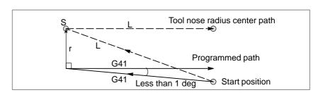
If the command is specified at start-up, the offset vector is not created.
