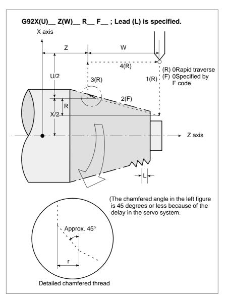
Fig. 13.1.2 (b) Taper thread cutting cycle
