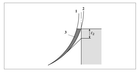
Although the tool should be positioned at 2 in the above figure, the tool is positioned at 1 (the tool nose is tangent to line L).
