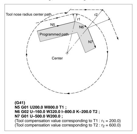
In the above example, the arc in block N6 is placed in the one quadrant. But after tool nose radius compensation, the arc is placed in the four quadrants.
