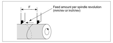
Fig. 5.3 (c) Feed per revolution
