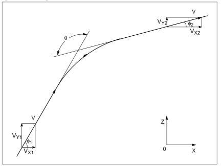
Fig. D.3 (b) Example of tool path
