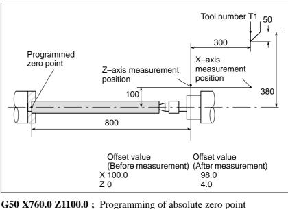
**GS0 X760.0 Z1100.0**; Programming of absolute zero point (Coordinate system setting) **S01 M03 T0101**; Specifies tool T1, offset number 1, and spindle revolution
