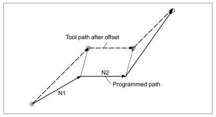
Fig. 14.1.5 (b) Movement of offset (2)
