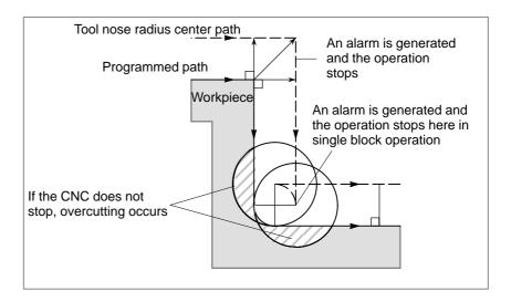
Machining a groove smaller than the tool nose radius Since the tool nose radius compensation forces the path of the center of the tool to move in the reverse of the programmed direction, overcutting will result. In this case an alarm is displayed and the CNC stops at the start of the block.
