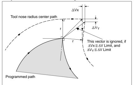
If  $\Delta Vx \leq \Delta V$  limit and  $\Delta Vy \leq \Delta V$  limit, the latter vector is ignored. The  $\Delta V$  limit is set in advance by parameter (No. 5010).
