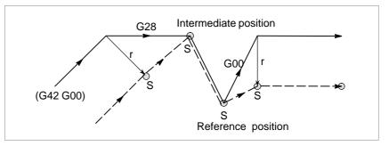
Tool nose radius compensation G code in the offset mode The offset vector can be set to form a right angle to the moving direction in the previous block, irrespective of machining inner or outer side, by commanding the tool nose radius compensation G code (G41, G42) in the offset mode, independently. If this code is specified in a circular command, correct circular motion will not be obtained.
