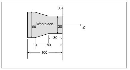
Fig. 1.3.2 (e) Coordinates and dimensions on part drawing
