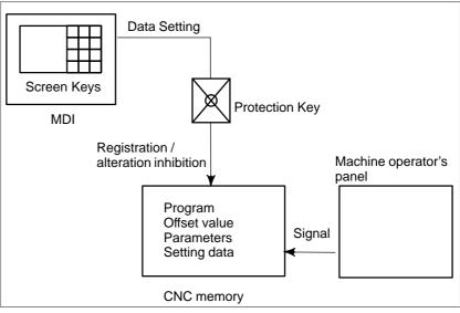
Fig. 1.6 (f) Data Protection Key
