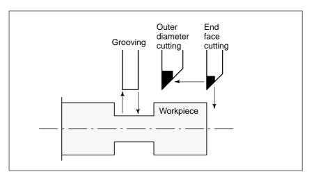
Prepare the program of the tool path and cutting condition according to the workpiece figure, for each cutting.
