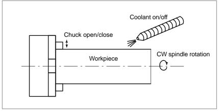
Fig. 1.6 Command for machine operations
