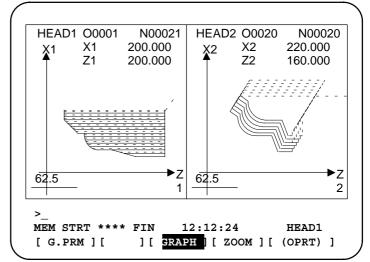
Parameter GRL (bit 0 of No. 6500) specifies which tool post is to be displayed on which side.
