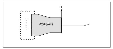
Fig. 1.3.2 (f) Coordinate system on lathe as specified by CNC (made to coincide with the coordinate system on part drawing)
