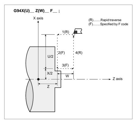
Fig. 13.1.3 (a) Face Cutting Cycle
