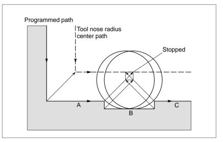
There is no actual interference, but since the direction programmed in block B is opposite to that of the path after tool nose radius compensation the tool stops and an P/S alarm (No. 041) is displayed.
