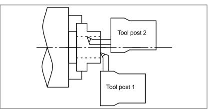
The contours of the two tool posts are checked to determine whether or not an interference occurs.
