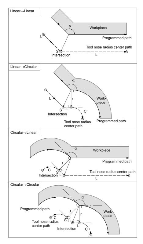
Tool movement around the outside corner at an acute angle (α<90°)</li>
