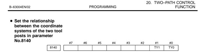
TY0, TY1:Set the relationship between the coordinate systems of the two tool posts, with tool post 1 used as the reference.
