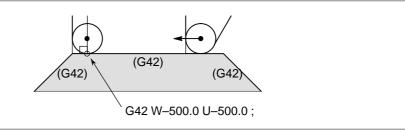
In the block that first specifies G41/G42, the above positioning of the tool nose center is not performed.
