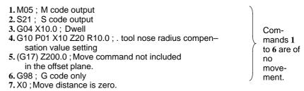
A block without tool movement specified in offset mode
