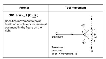
Fig. 13.5 (a) Chamfering ( $Z \rightarrow X$ )
