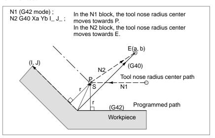
In this case, note that the CNC obtains an intersection of the tool path irrespective of whether inner or outer side machining is specified
