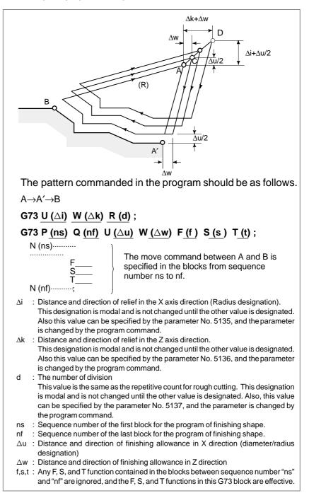
Fig. 13.2.3 Cutting path in Pattern Repeating
