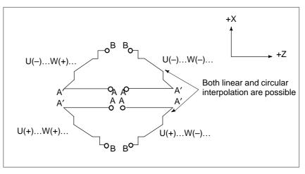
Fig. 13.2.2 (b) Signs of Numbers Specified with U and W in Stock Removal in Facing
