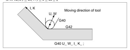
Tool movement when the moving direction of the tool in a block which includes a G40 command is different from the direction of the workpiece
