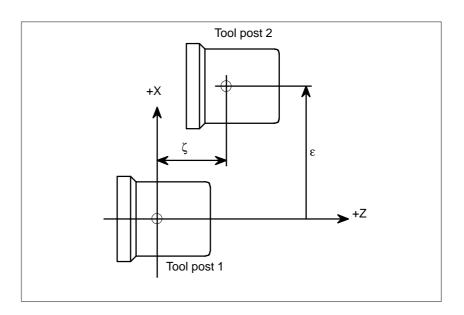
In the ZX plane coordinate system at the origin of which the reference point of tool post 1 is set, set the X coordinate ( $\epsilon$ ) of the reference point of tool post 2 in parameter No. 8151, and its Z coordinate ( $\zeta$ ) in parameter No.8152.
