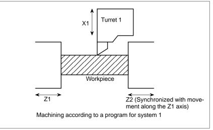
Synchronizes movement along an axis of one system with that along another axis of the same system.
