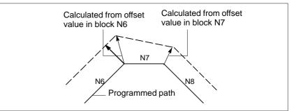
When some vectors are produced between blocks N6 and N7, the vector at the end point of the present blocks is calculated using the offset value of the block N6.
