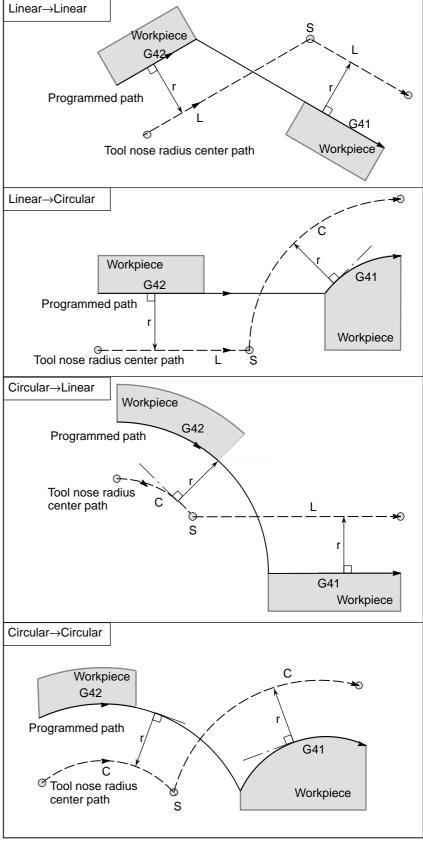
Tool nose radius center path without an intersection When changing the offset direction in block A to block B using G41 and G42, if intersection with the offset path is not required, the vector normal to block B is created at the start point of block B.
