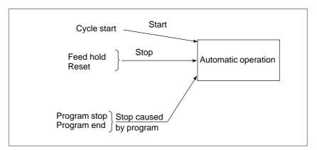
Fig. 1.3 (b) Start and Stop for Automatic Operation
