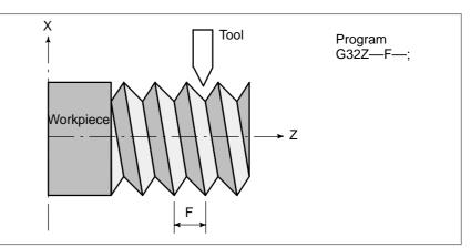
Fig. 1.1 (e) Straight thread cutting
