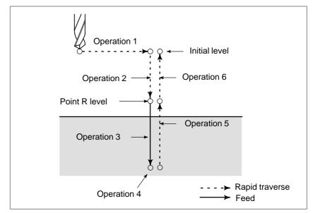
Fig. 13.3 Drilling Cycle Operation Sequence
