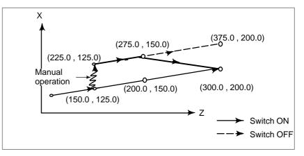
Manual operation after the end of block  When reset after a manual operation following a feed hold Coordinates when the feed hold button is pressed while block (2) is being executed, manual operation (Y-axis+75.0) is performed, the control unit is reset with the RESET button, and block (2) is read again
