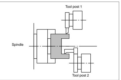
Fig. 20.1 (a) Application to lathes with one spindle and tow tool posts
