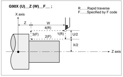
Fig. 13.1.1 (a) Straight Cutting Cycle
