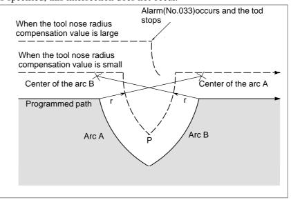
• The center of the arc is identical with the start position or the end position
