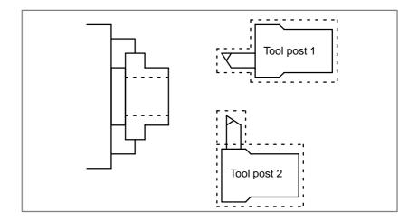
When interface forbidden areas (tool shapes) as indicated by dashed lines are set for tool posts 1 and 2 as shown above, a check is made by determining whether the two interference forbidden areas indicated by dashed lines overlap each other after the movement of the tool posts.
