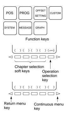
The function keys are used to select the type of screen (function) to be displayed. When a soft key (section select soft key) is pressed immediately after a function key, the screen (section) corresponding to the selected function can be selected.
