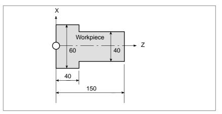
Fig. 1.3.2 (c) Coordinates and dimensions on part drawing
