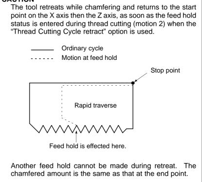
• Taper thread cutting cycle
