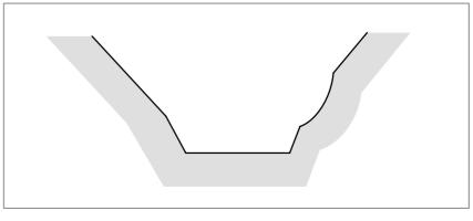
Fig. 13.2.1 (d) Figure Which Can Be Machined (Monotonic change) in Stock Removal in Turning (Type II)
