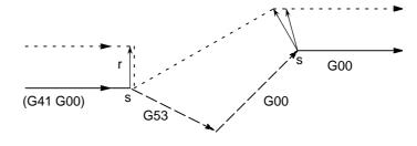
Example 2) When bit 2 (CCN) of parameter No. 5003 is set to 1 and all-axis machine lock is applied
