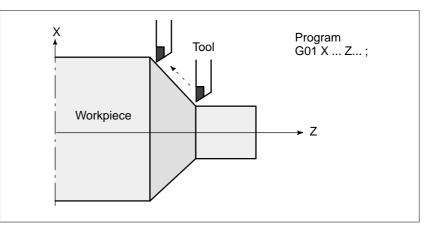
Fig.1.1 (b) Tool movement along the taper line
