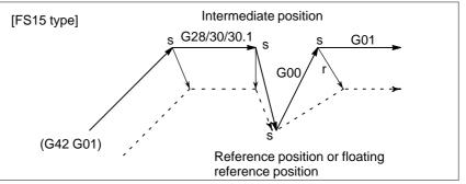
G28, G30, or G30.1 command in offset mode (with movement to an intermediate position not performed)
