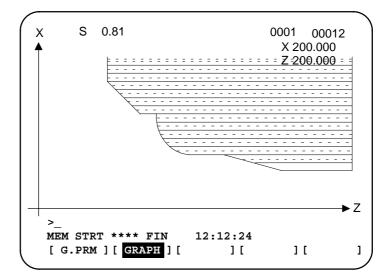
**12** To display the original drawing, press the **[NORMAL]** soft key, then start automatic operation.
