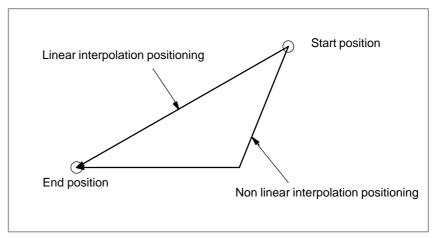
The rapid traverse rate in the G00 command is set to the parameter No. 1420 for each axis independently by the machine tool builder. In the positioning mode actuated by G00, the tool is accelerated to a predetermined speed at the start of a block and is decelerated at the end of a block. Execution proceeds to the next block after confirming the in–position.
