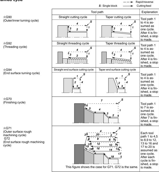
Fig. 5.5 Single block during canned cycle (1/2)
