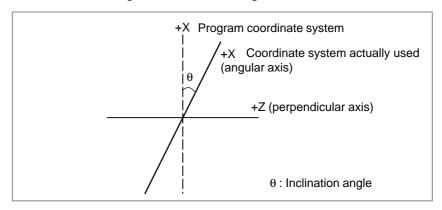
When the angular axis is the X-axis and the perpendicular axis is the Z-axis, the amount of travel along each axis is controlled according to the formulas shown below.
