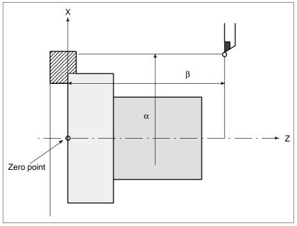
Fig. 7 Tool Position Specified by  $X\alpha Z\beta$
