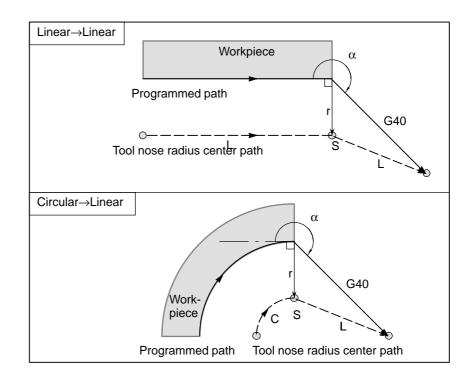
Tool movement around an outside corner at an obtuse angle (90° ≦ α<180°)</li>
