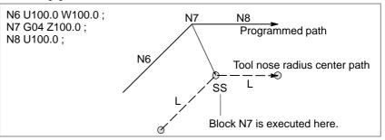
However, when the move distance is zero, even if the block is commanded singly, tool motion becomes the same as that when more than one block of without tool movement are commanded, which will be described subsequently.
