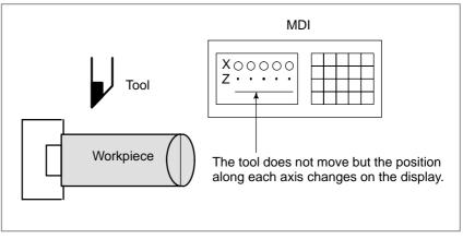
Fig. 5.1 Machine lock
