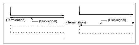
2. When the tool cuts a workpiece along the X-axis, if a skip signal is input, the tool stops cutting immediately and returns to the Z coordinate where the cycle started.
