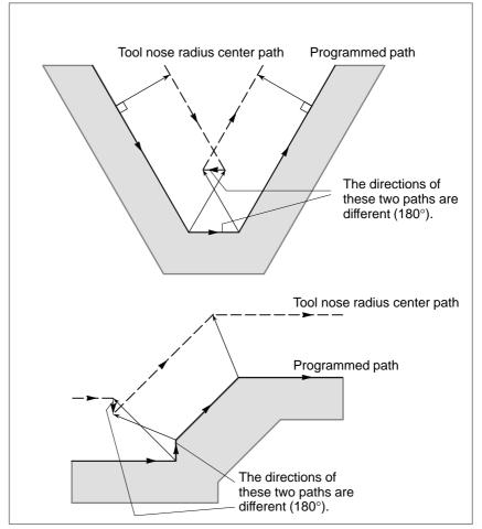
(2) In addition to the condition (1), the angle between the start point and end point on the Tool nose radius center path is quite different from that between the start point and end point on the programmed path in circular machining(more than 180 degrees).
