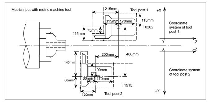
The coordinate systems shown on the right of the figure above are the ZX plane coordinate systems of tool posts 1 and 2. For clarity, the coordinate systems are shifted; actually, the origins of the coordinate systems must match the machine zero points.
