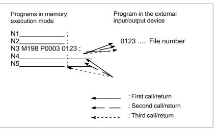
Fig. 4.5 Program Flow When M198 is Specified
