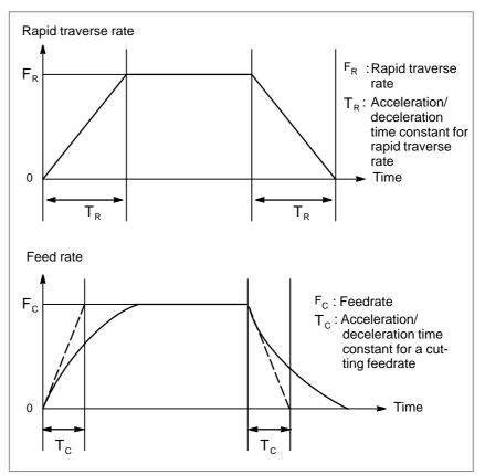
Fig. 5.1 (a) Automatic acceleration/deceleration (example)
