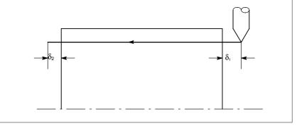
Fig. D.2 Incorrect threaded portion
