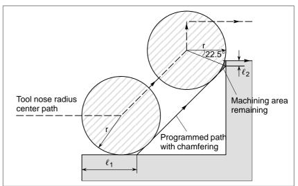
The following example shows a machining area which cannot be cut sufficiently.
