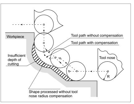
Fig 14.2 Tool path of tool nose radius compensation
