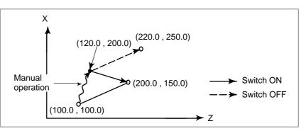
Manual operation after a feed hold Coordinates when the feed hold button is pressed while block (2) is being executed, manual operation (X-axis + 75.0) is performed, and the cycle start button is pressed and released
