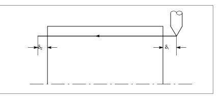
Fig. D.1 (a) Incorrect thread position
