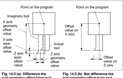
tool geometry offset from tool wear offset
