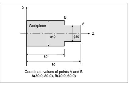
Fig. 1.3.3 (c) Diameter programming
