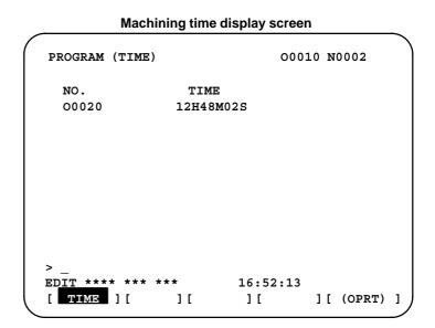
**5** To calculate the machining times of additional programs, repeat the above procedure. The machining time display screen displays the executed main program numbers and their machining times sequentially.
