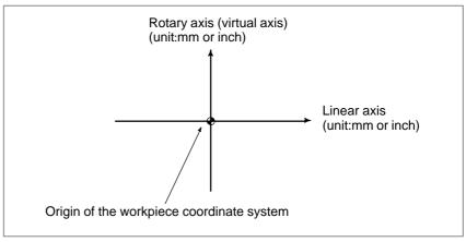
Fig. 4.5 (a) Polar coordinate interpolation plane.
