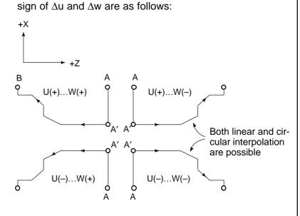
The tool path between A and A' is specified in the block with sequence number "ns" including G00 or G01, and in this block, a move command in the Z axis cannot be specified. The tool path between A' and B must be steadily increasing or decreasing pattern in both X and Z axis. When the tool path between A and A' is programmed by G00/G01, cutting along AA' is performed in G00/G01 mode respectively.
