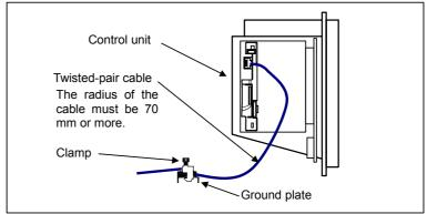
The Ethernet cable must be fastened by a cable clamp to prevent tension being applied to the modular connector (RJ-45) that connects the cable to the control unit even if the Ethernet cable is pulled directly. This clamp is also used to ground the cable shield.
