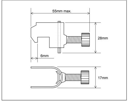
External dimensions of clamp fixture
