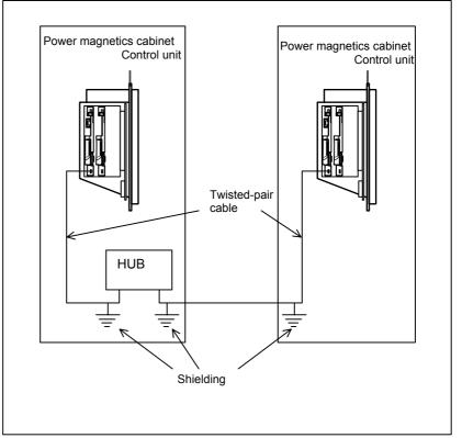
Example of shielding of transceiver cable
