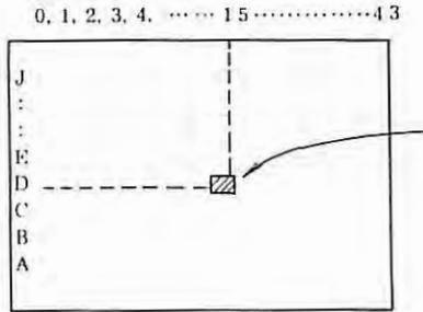
These addresses are marked with 0 - 43 in the horizontal direction and with A - J numbers in the vertical direction of PCB.
