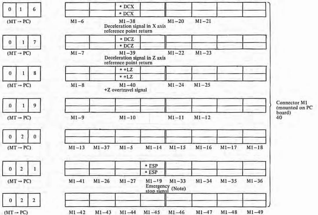
Note) Bit 4 in DGN No. 21 and bit 4 in DGN No. 101 are effective as emergency stop signal when PC-MODEL D, MODEL H are provided.
