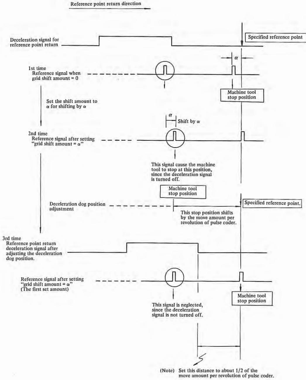
Fig. 7.5.5(a) Adjustment of Operating Position of Reference Point Return (Grid system)
