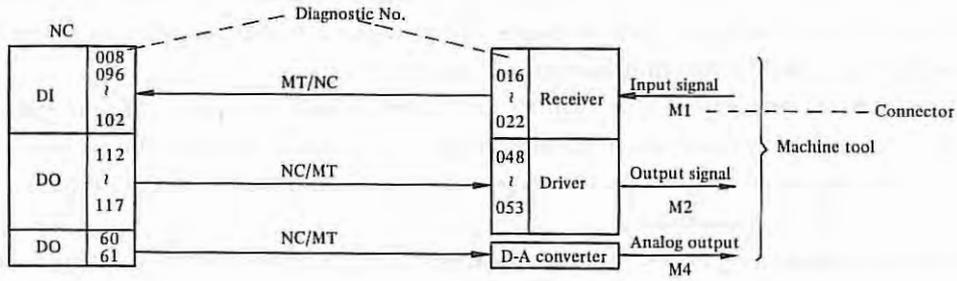
An I/O signal is read out with the same content for DGNOS No. 096-102 and 016-022 and also for 122-117 and 048-053.
