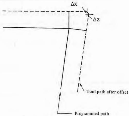
If X CRCDL and Z CRCDL, the small movement is ignored. This prevents the workpiece from being affected by stopping the tool at the corner.
