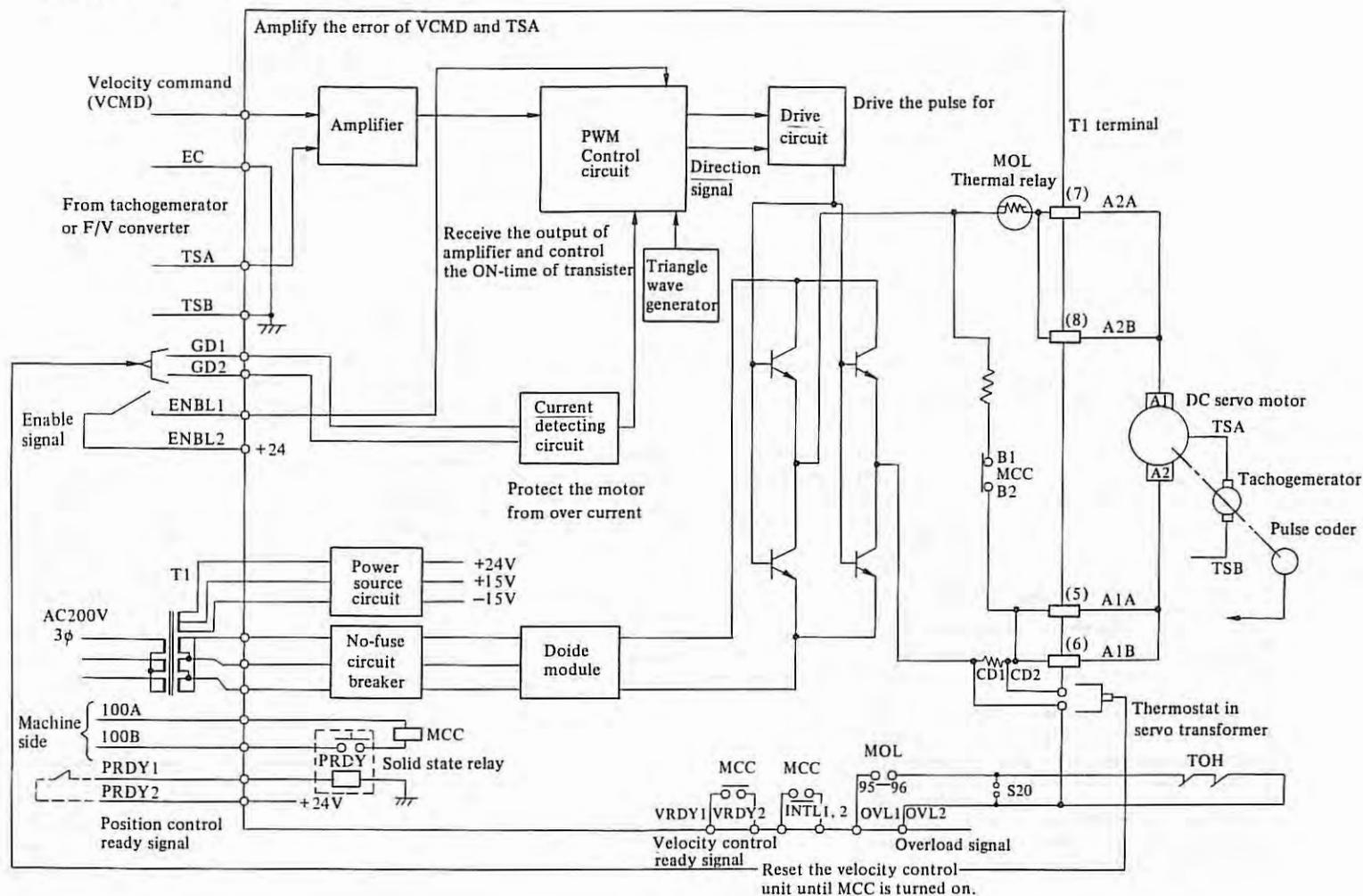
(Note) Open-circuit at S20 for velocity unit which is connected to servo transformer.
