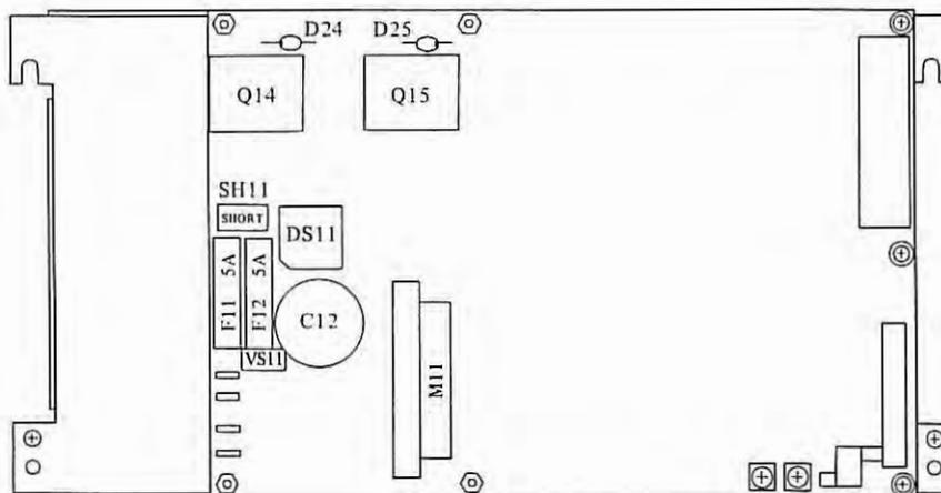
Arrangement of main parts of primary circuit (with the cover removed)
