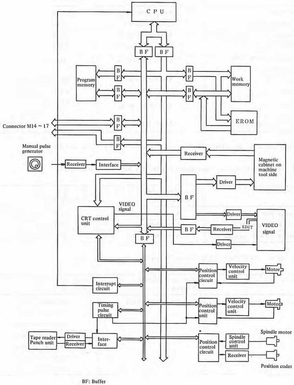
Fig. 1.1(e) System Configuration
