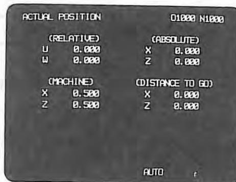
(MACHINE) Shows the machine tool position from the reference point.
