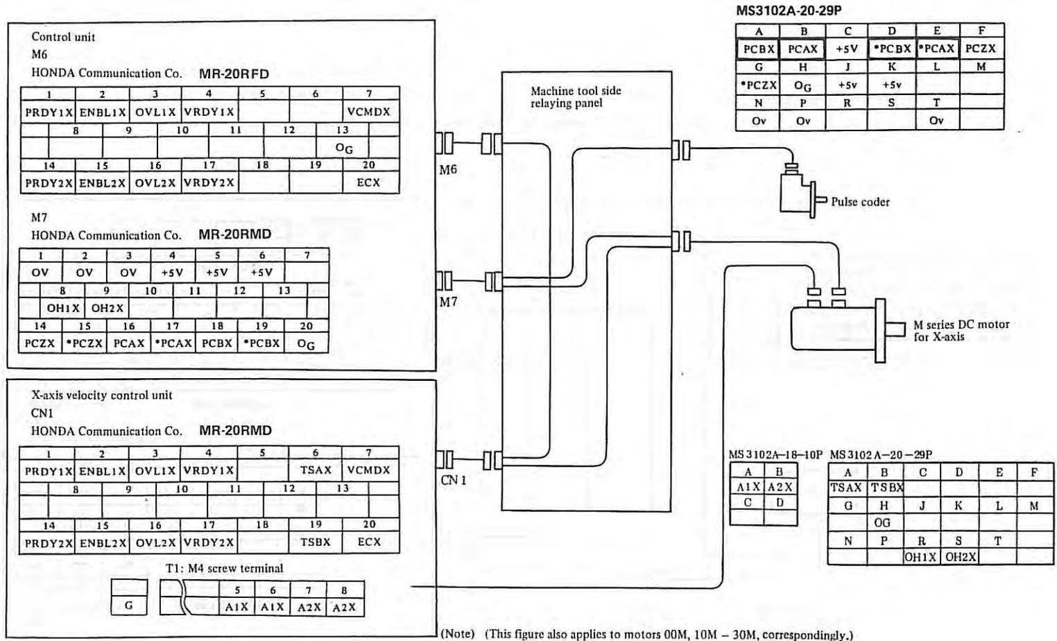
Fig. 1(b) Connection of Motor Model 0M and 5M
