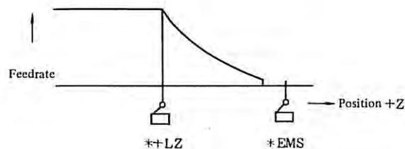
\*+LZ operation ..... The machine tool is decelerated and stopped with OVERTRAVEL displayed on the display unit.
