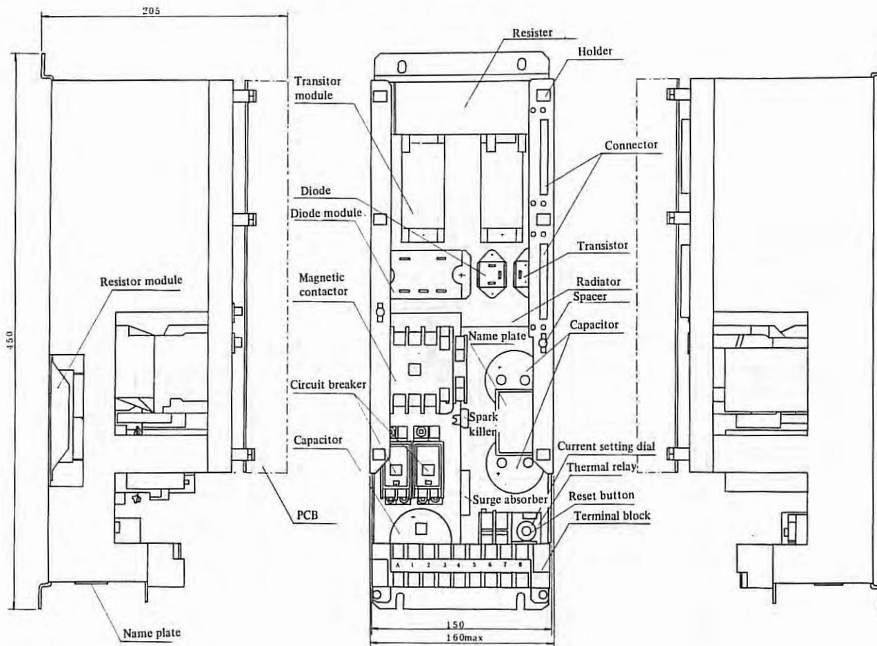
5.2.4 Velocity control unit for MODEL 30M (A06B-6047-H004)
