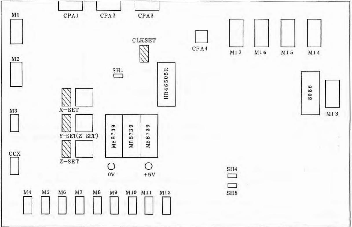
Fig. 4.1 Set Points of Master PCB (A16B-1000-0010)
