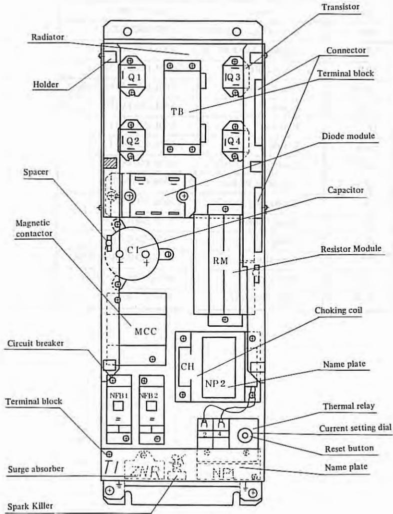
5.2.3 Velocity control unit for MODEL 10M, 20M (A06B-6047-H003)
