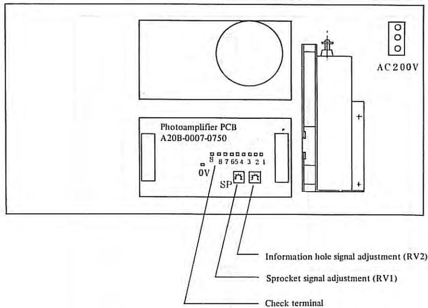
Note) For adjusting the output waveform of the photoamplifier, use a blue, white, pink, or yellow tape other than black and gray tapes. If a blue, white, pink or yellow tape is loaded to the tape reader which has been adjusted by using a black or gray tape, an error is produced. Don't adjust the tape reader by using a black or gray tape. (If a black tape only is used at all times, the tape reader may be adjusted by using the black tape.)
