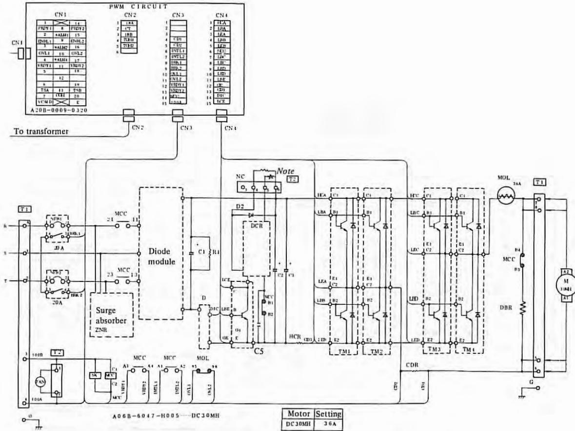
Note) Remove the short bar when the discharge unit is provided.
