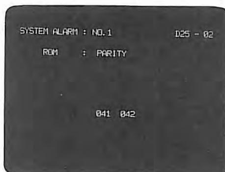
The display of the CRT of the FS 3T-C and that of FS 2T-A is a little different.
