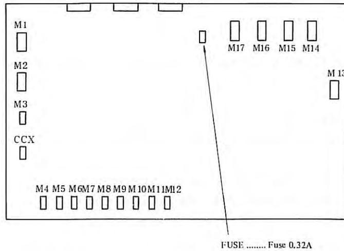
Fig. 1.1(c) Mounting Position of Master PCB Fuse
