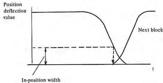
In-position check is performed when the feed mode changes from rapid traverse to rapid traverse, rapid traverse to cutting feed, or cutting feed to rapid traverse.
