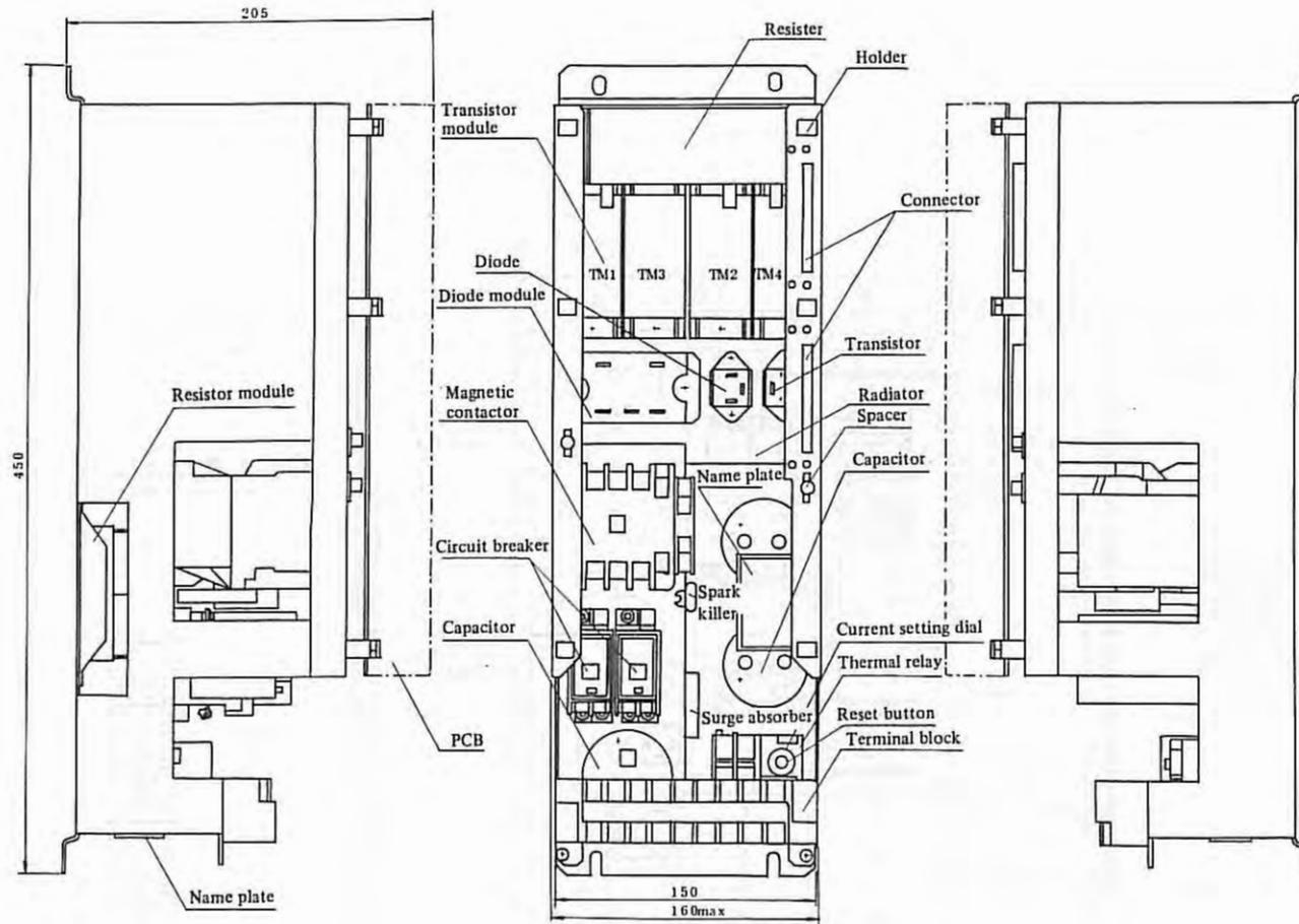
5.2.5 Velocity control unit for MODEL 30MH (A06B-6047-H005)
