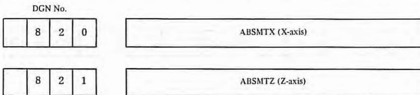
The machine tool position from the reference point is also displayed on the position display page of CRT character display unit.
