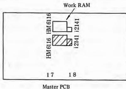
The shadowed part shows the low byte part, and the other shows the high byte part. (See 1.4.4)
