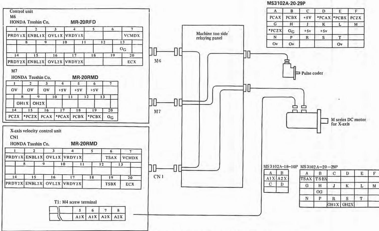
(Note) (The figure also applies to motors 00M, 10M - 30M, correspondingly.)
