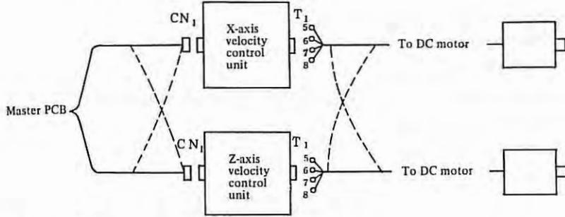
Exchange cables to velocity control unit CN1.
