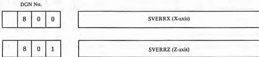
The position deviation amounts of X-axis and Z-axis are sequentially displayed.
