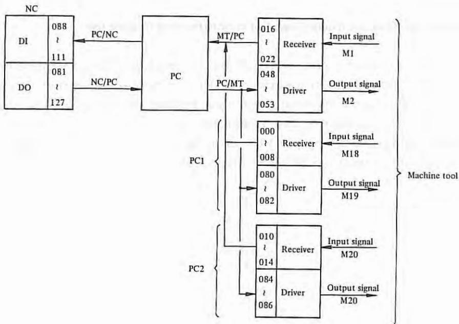
When I/O signals have been read, data of DGN No. 088 - 111 are the same as those of DGN No. 016 - 022. Also, read data of DGN No. 081 - 127 are the same as those of DGN No. 048 - 053.
