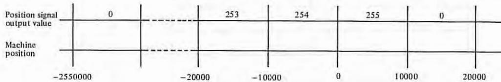
Note) Grid No. at the reference point is set by parameter No. 1046, 1047.
