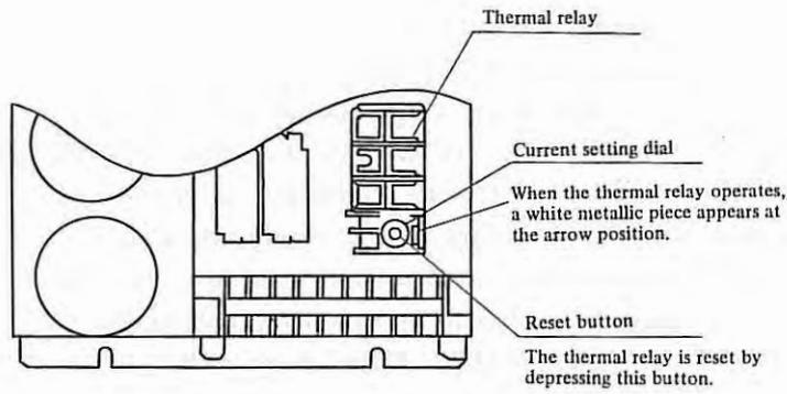
Fig. 7.4.11(b) Mounting Position of Thermal Relay for Motor Model 30MH
