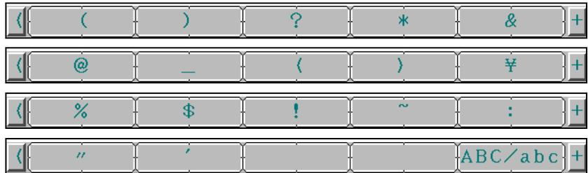
Pressing soft key [ABC/abc] switches between uppercase and lowercase characters for input. Which case can be currently input is indicated in the key input field.
