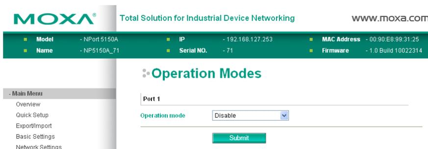
When Operation mode is set to Disabled, that particular port will be disabled. Check the "Apply the above settings to all serial ports" to apply this setting to the other port.
