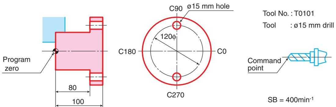
To drill two 15 mm dia. holes, create a program as indicated below:
