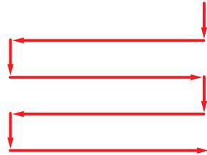
Cutting direction changes along the cutting path
