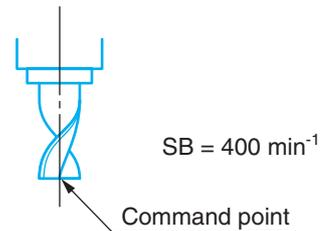
When cutting a thread having a width of 5 mm and 60 mm long as shown above, program as below using G185 to call out the thread cutting fixed cycle.
