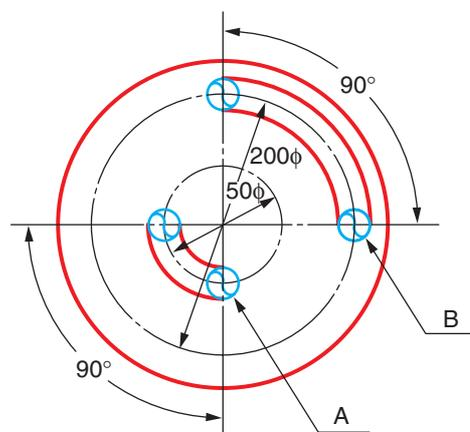
Axis movement distance along slot A:  $\dots\dots\dots\pi \times 50/4 \approx 39$  mm
