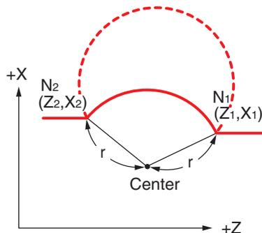
To move the tool along the arc indicated by dashed lines, program as follows:
