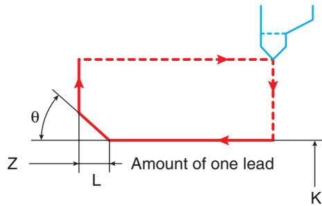
Equal to one lead when no L command is given
