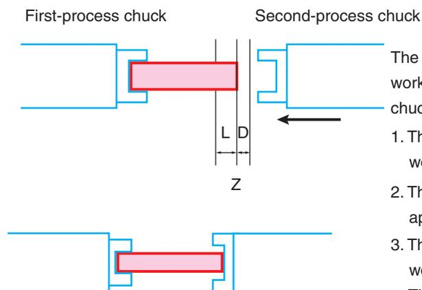
The explanation here is for a case in which a workpiece is transferred from the first-process chuck to the second-process chuck.
