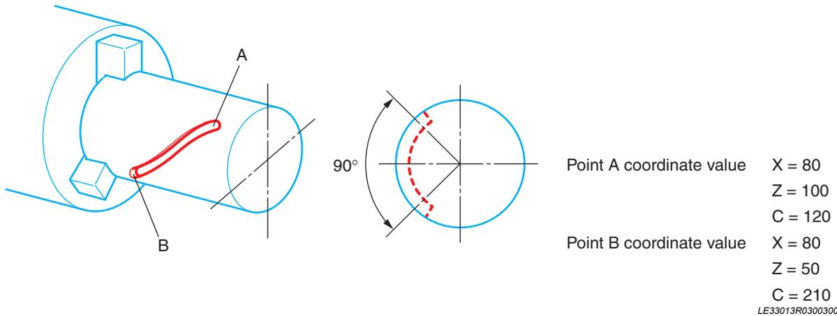
When cutting the spiral from A to B with a two-flute end mill under the following cutting conditions, calculate the feedrate of C-axis as explained below:
