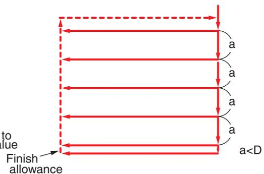
Infeed amount "a", obtained by dividing the total depth of cut to the target point into equal parts is determined so that "a" is not greater than "D".
