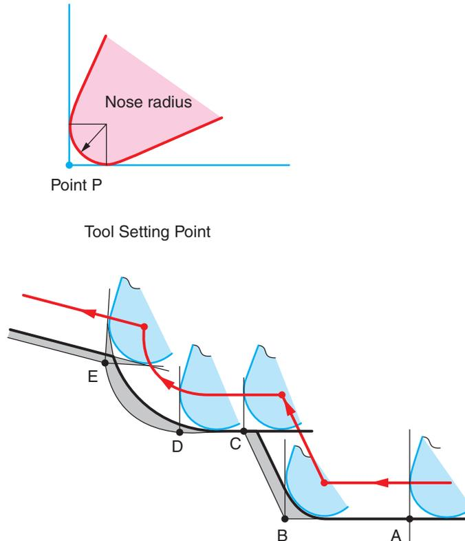
Tool Path and Resulting Error Without Tool Nose Radius Compensation
