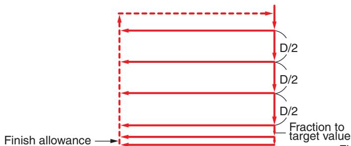
The tool is infeed by the designated amount "D"; in the final cutting path, the depth equivalent to the fraction is cut.
