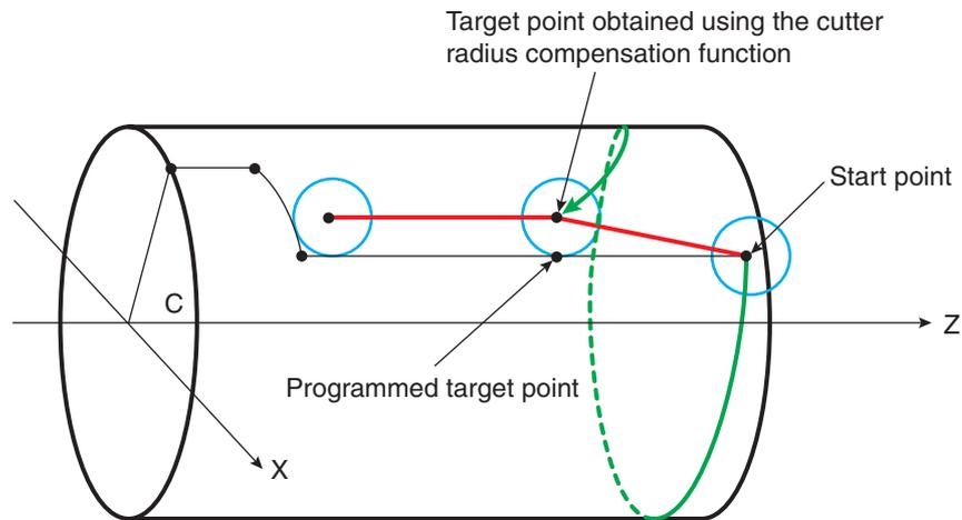
Cutter Radius Compensation for Contour Generation (Side) (2/2)
