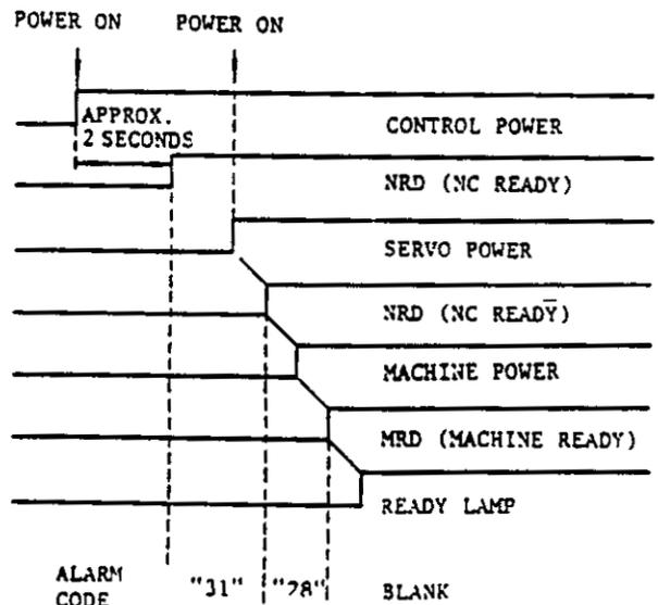
Fig. 4.2.1 Sequence of Turning on Operation
