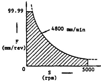
Fig. 2.5.1.1 Restriction of Feedrate and Spindle Speed
