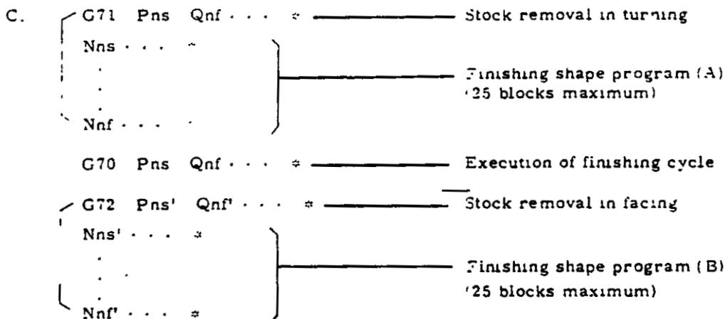
After executing the above program the program (A) is eliminated and the program (B) is retained in the finishing shape memory. Therefore, the finishing command with G70 in the trailing program is effective for the finishing shape program (G).
