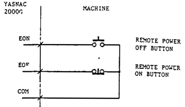
Fig. 4.2.3 Connections of Remote Power ON/OFF Buttons
