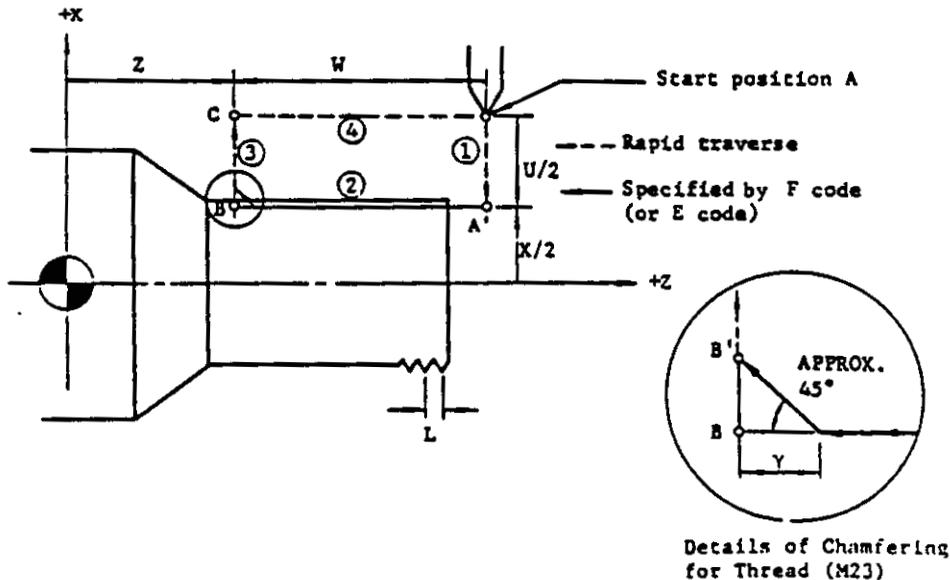
Details of Chamfering for Thread (M23)
