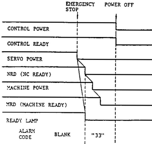
Fig. 4 2.2 Sequence of Turning Off Operation
