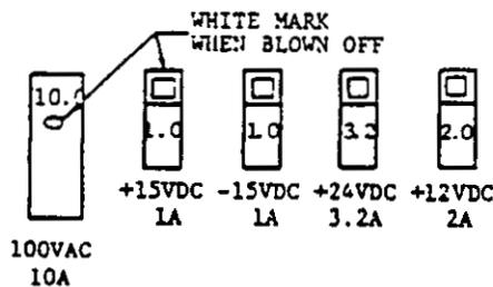
Fig. 8.3.1 Fuses of Composite Control Power Supply Unit
