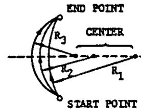
Therefore, in the following case, the arc center does not exist which causes data error.
