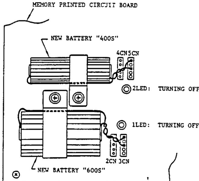
Fig. 8.2.2 Arrangement of Replaced Battery
