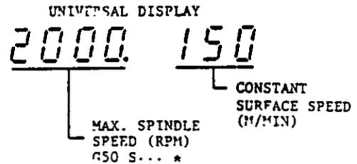
Fig. 4.3.1.3 Example of All S-codes Display
