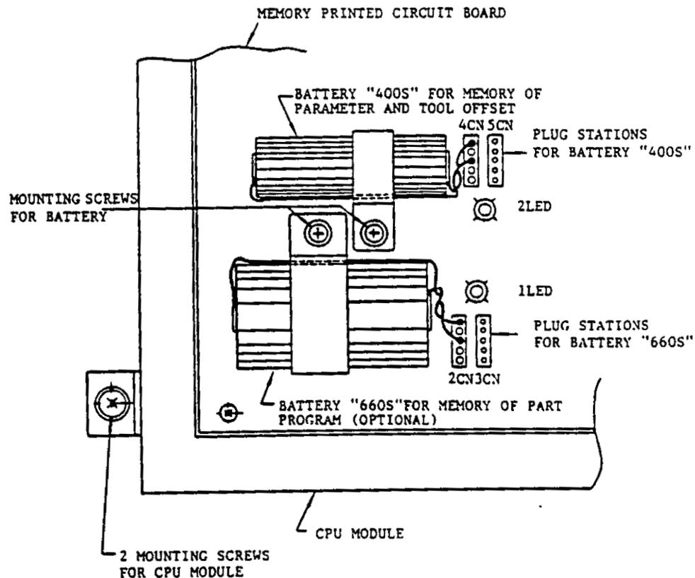
Fig. 8 2.1 Arrangement of LED and Battery
