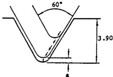
Depth of cut for each cycle when a (fixed amount) is 0.2 mm
