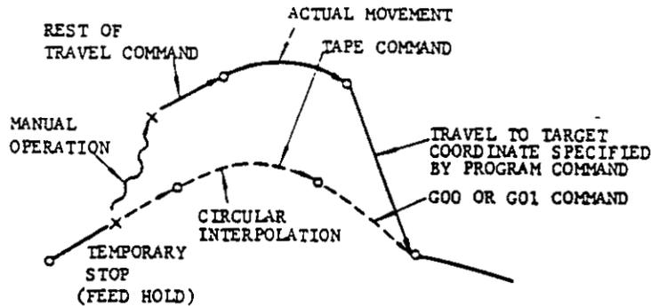
Fig. 6.1.18.1 Tool Movement with MANUAL ABSOLUTE Switch On
