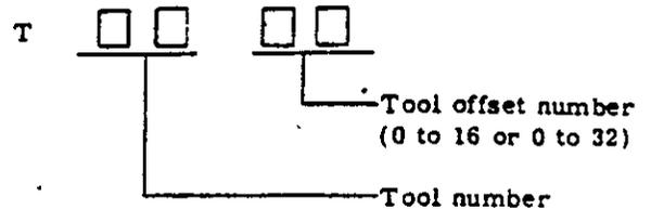
The figures usable for the designation of tool number are determined by the machine. Refer to the machine tool builder's manual.
