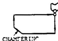
When M23 is commanded before the command of threadcutting cycle G92 (or G76<sup>+</sup>), chamfering of thread is performed. If M24 is commanded, chamfering with threadcutting is not performed.
