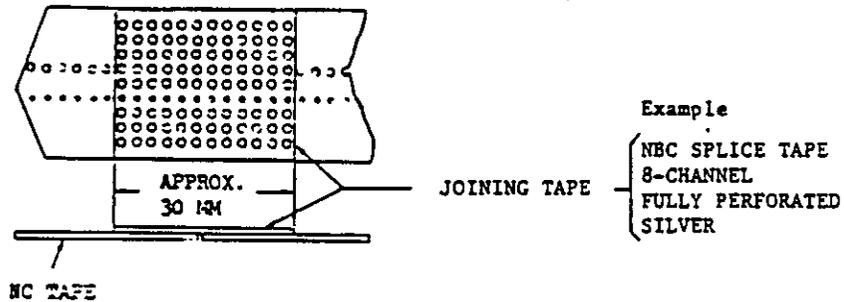
Fig. 3.4.1 Splicing of NC Tape
