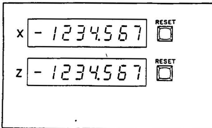
Fig. 4.3.16 Current Position Display Unit
