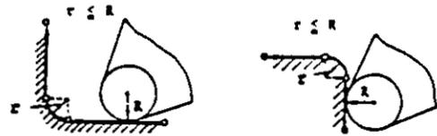
(Compensation for inside of circular arc) (a) Error
