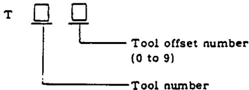
The figures used for the designation of tool number are determined by the machine. Refer to the machine tool builder's manual.
