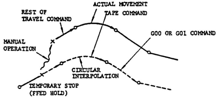
Fig. 6.1.18.2 Tool Movement with MANUAL ABSOLUTE Switch Off
